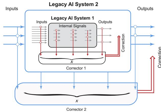
**Fig. 2.** Cascade of AI correctors. In this diagram, the original legacy AI system (shown as Legacy AI System 1) is supplied with a corrector altering its responses. The combined new AI system can in turn be augmented by another corrector, leading to a cascade of AI correctors.
