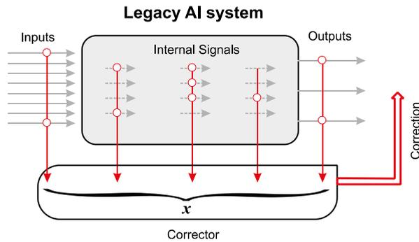
Fig. 1. Corrector of AI errors. Inputs for this corrector may include input signals, and any internal or output signal of the AI system (marked by circles).
